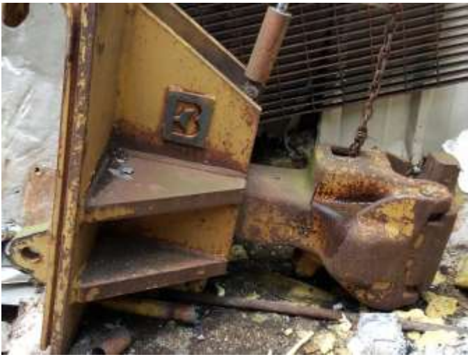
211. Rail car coupler for High Loader to move rail cars
